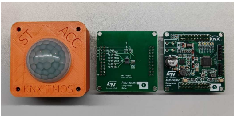
TMOS sensor with KNX-TP
