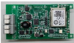
KNX-LoRa project based on STM32WL STKNX
